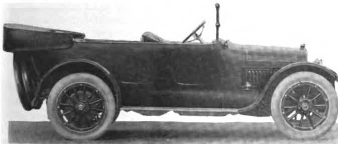
1916 Cadillac seven-passenger touring car. Note straight top line. There is a new mud flap in front below the radiator protecting the water pumps from splash
